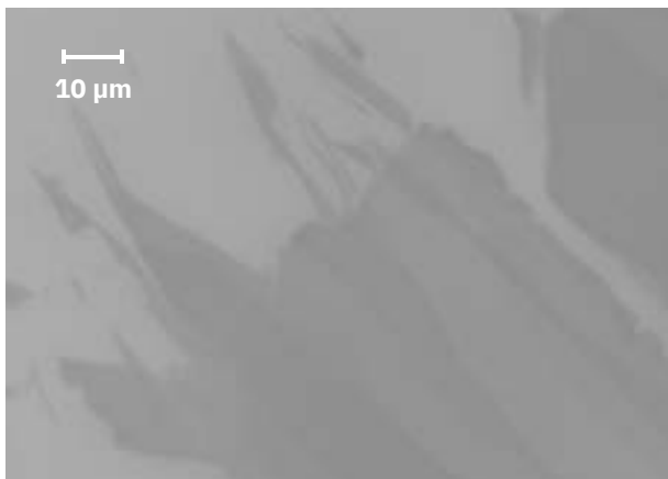
SEM secondary electron image of graphene corresponding to the same area as the Raman images shown.
