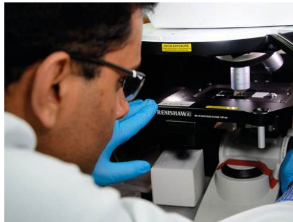
Raman spectrometer in action
